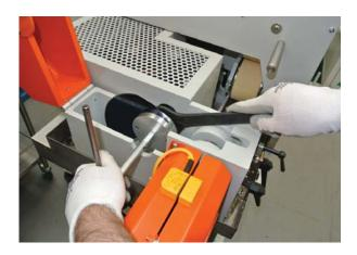
8) Remove the blade locking bolt, washer & blade cap.
