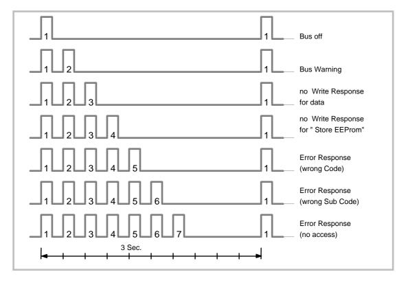
Errors 2...7 can be reset by pressing the Enter button. To reset Error 1 it is necessary to switch off the unit and power up again.
