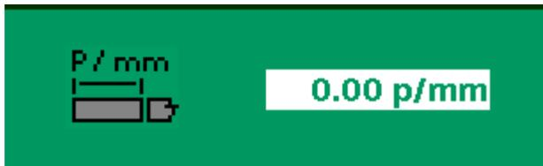
Adjusts scaling factor to adjust entered cut length on HMI and actual length. Factory set
