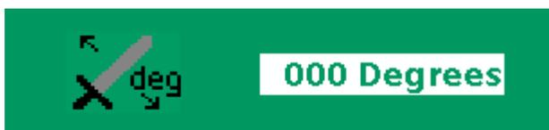
Adjusts blade datum (stop position) in single blade mode. Factory set to 180' from cut point
