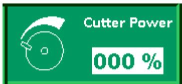
Adjust blade power in on demand mode. 100% = 2000 RPM.
