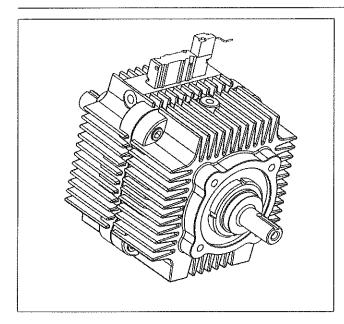
EasyStep generates cyclic stop/go motions via reciprocal clutching and braking actions while the driving motor operates at constant speed.
