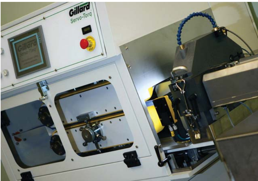
△ The digital camera is integrated into a Servo-Torq® Plus LT rotary cutter with combined Accra-Feed™ caterpillar infeed.
