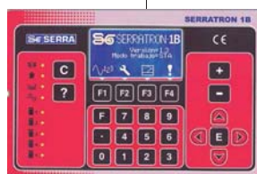
The Weld Control Screen :
